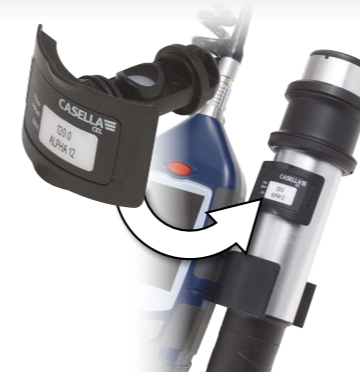
On-site calibration device
